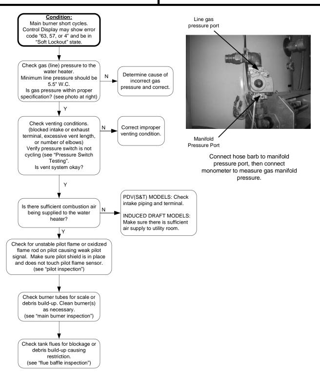
Main Burner & Pilot Removal and Inspection
